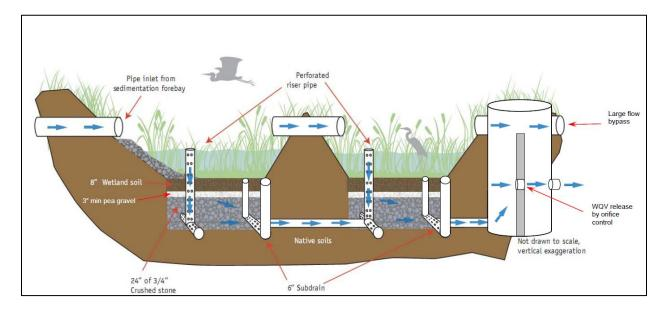
Schematic of a subsurface gravel bed wetland from the University of New Hampshire Stormwater Center Design Criteria (University of New Hampshire Stormwater Center (UNHSC), 2009).
