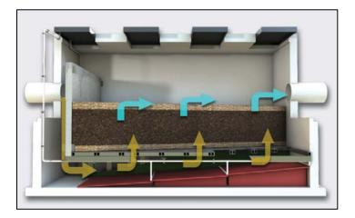
Schematic of the Nutrient Removing Filtration System® by SunTree (SunTree Technologies Inc., 2020). **Figure 5-8** Schematic of the Nutrient Removing Filtration System®
