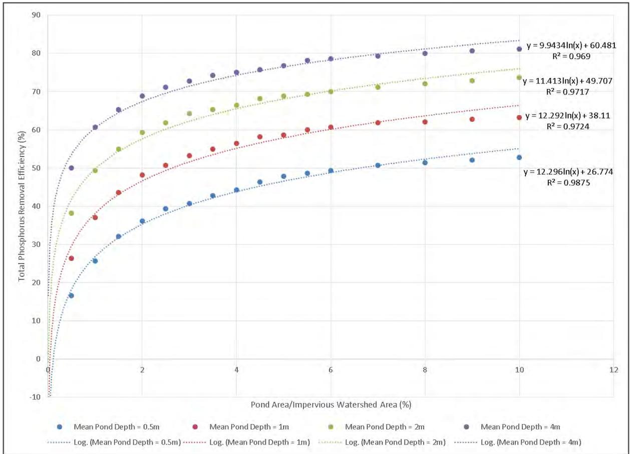
Figure A.1 Curves relating detention pond surface area, watershed impervious area, pond depth, and total phosphorus removal efficiency
