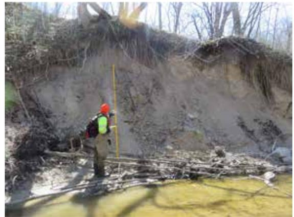
*Measuring severe bank erosion along Bluff Creek*
