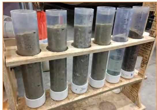
**Figure 4-27 Spent Lime/Sand Mixture Column Testing**
