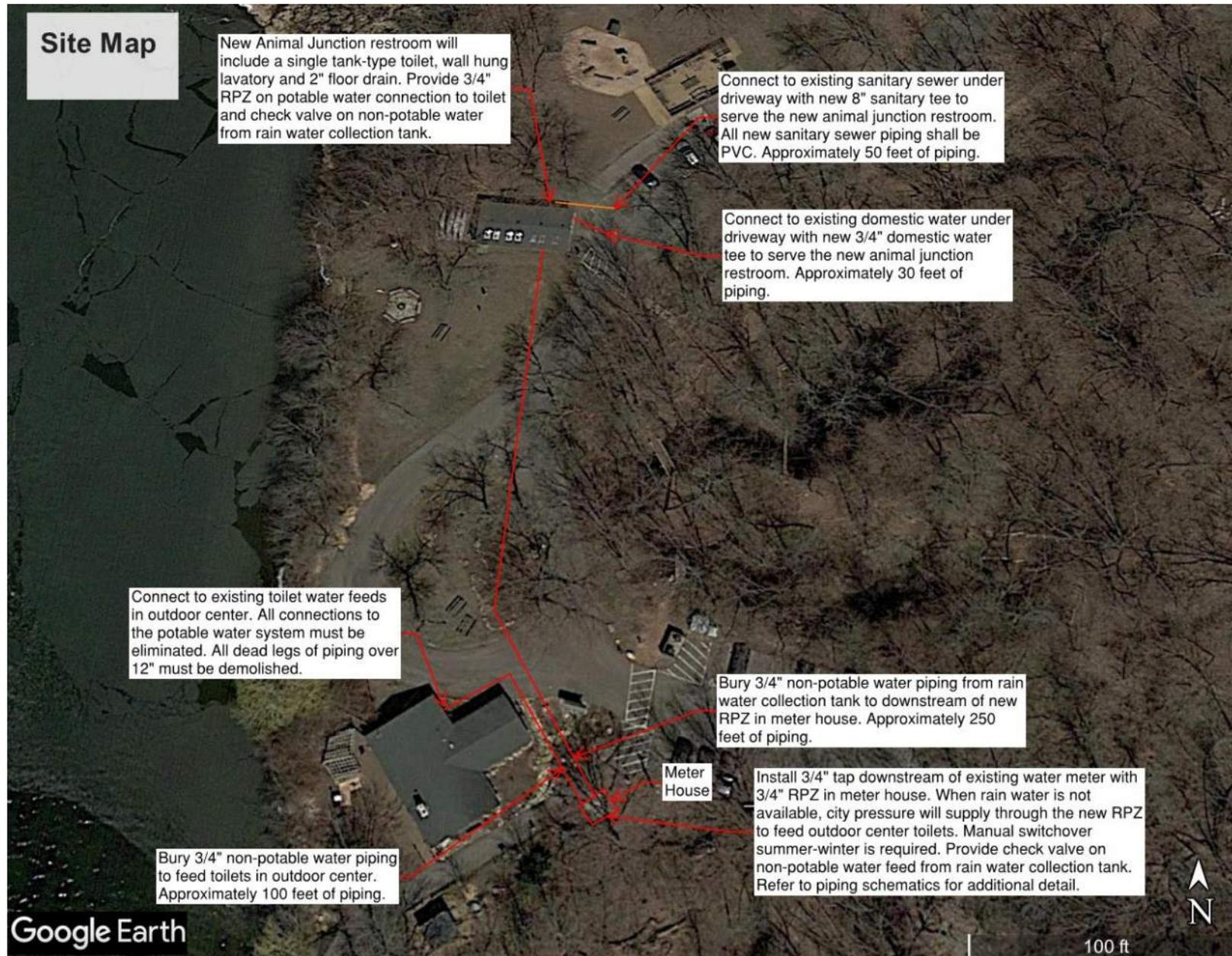
Figure 3. Preliminary Site Plan for Alternative 2.
