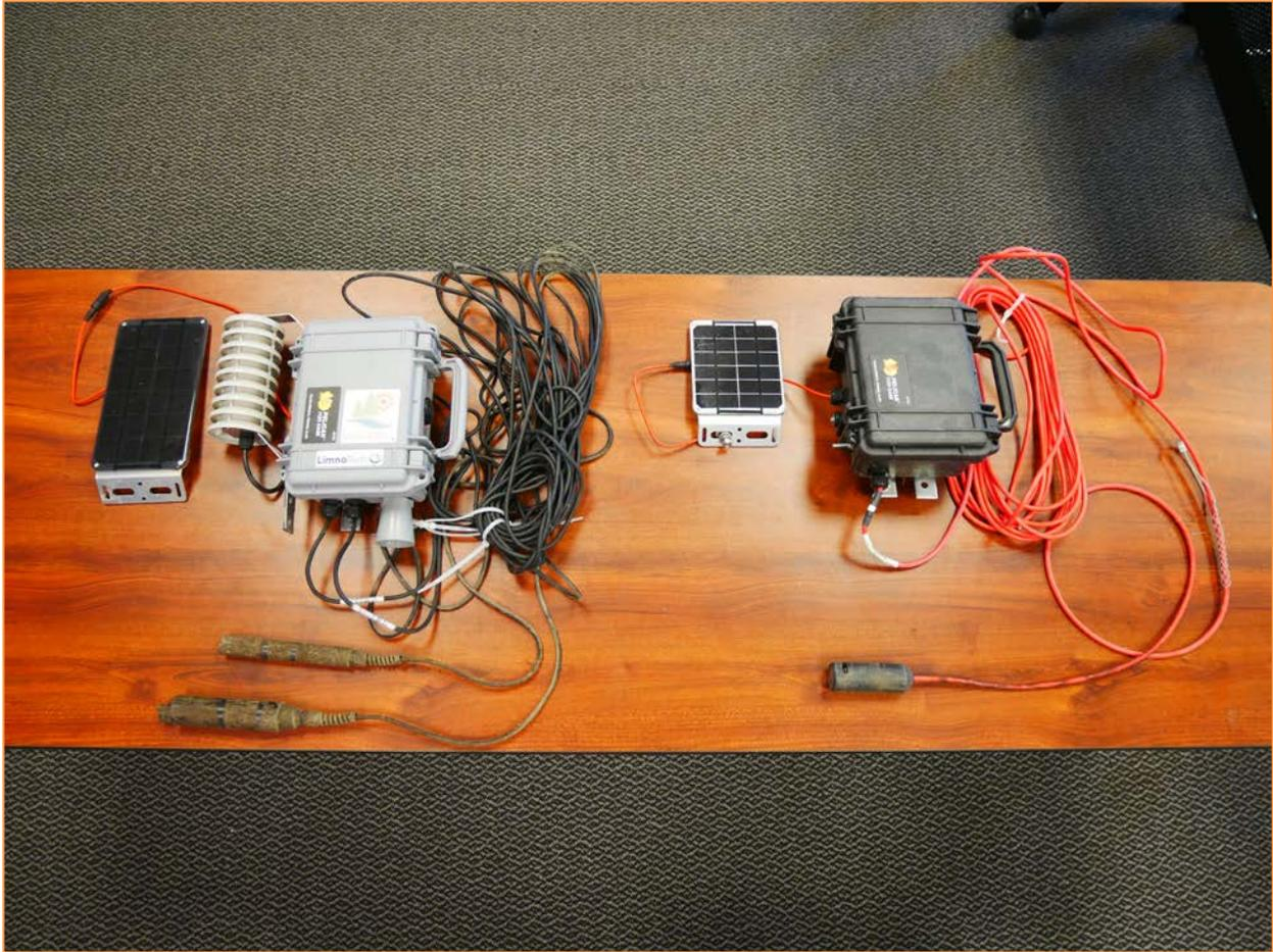
**Figure 4-33 EnviroDIY Water Monitoring Stations**
