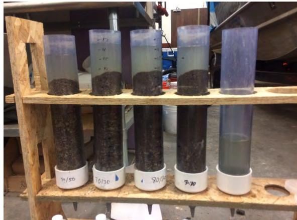
**Figure 1. Laboratory column testing of filter media completed by District staff during the summer of 2019.**
